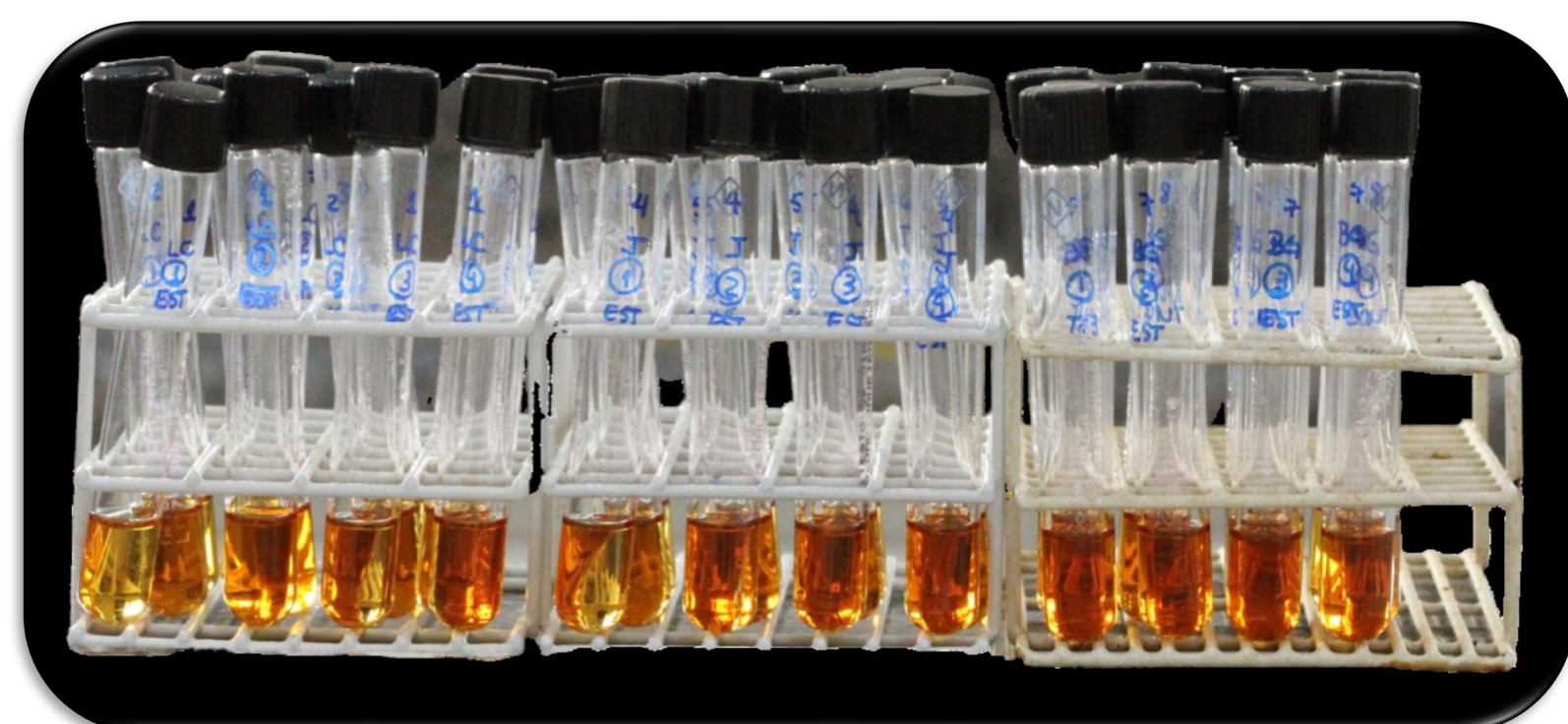
Fig. 1 Test tubes with membranes immersed for 7 days, in an incubator at 37°C. Groups C and aPDT (culture medium with oral biofilm); Group S (sterile culture medium).
